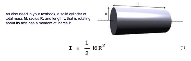
Note that I does not depend on the length L, so Eqn. 1 is also true for a thin disc of negligible thickness.
