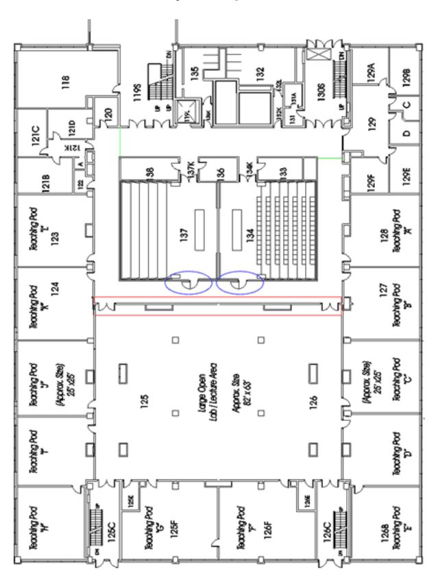
I made some modifications to Larry's plan. If we take the doors at the back of Rooms 134 and 137, which are circled in blue, and convert them to *Emergency Only*, then we can remove the wall that I have outlined in red. Then the entrance to the lab could be placed somewhere like the green lines in the above diagram.
