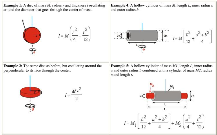
Figure 1. The equations of moments of inertia for the four objects used. [1]
