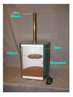
Figure 2. The apparatus used to measure the objects' period of oscillation. [1]
