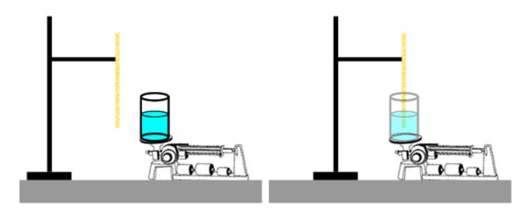
Above, the figure to the left shows a beaker of water on the pan of a balance. The balance is adjusted so that it reads the mass of the beaker and the water. To the left of the balance is a stand holding a piece of wooden dowel.
