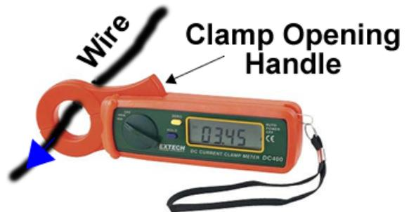
The jaws may be separated by pressing on the **Clamp Opening Handle**.
